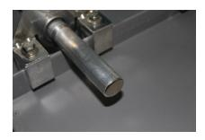
5. Slide Swaged Tube end into unfinished end of adjacent tubes to complete run.
