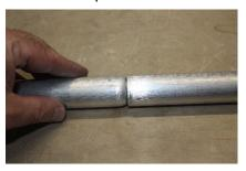
6. Slide End Collars onto tubing and tighten, being careful to locate the collars on the INSIDE of the last bracket in a run.
