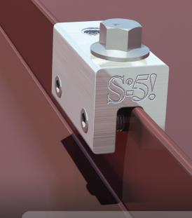
The S-5-E clamp is secured with our patented round-point setscrews without piercing the metal roof panel, thereby preserving the roof manufacturer's warranty!
