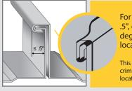
For horizontal seams under .5", crimp the seam to 180 degrees at desired clamp location.
