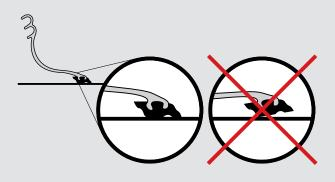
**Note:** SnoClip should not be used with Brass SnoFence and SnoRail™ on copper roofs.
